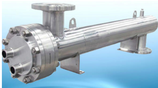
Sanitary U-tube Heat Exchanger with Double Tubesheets and Tri-clamp Fittings on Tube-side connections
